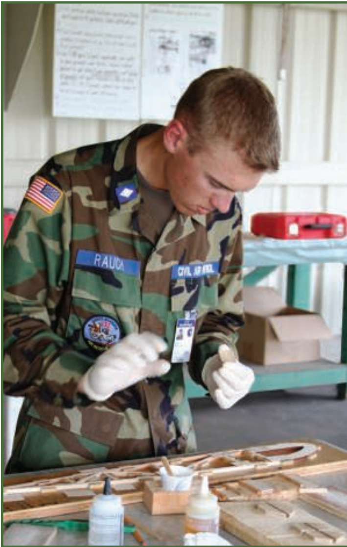
Cadet Maj. Ehren Rauch participates in one of Blue Beret's activities for cadets, building wing ribs.
